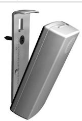
The optional transmitter mounting plate hinges to the transmitter. Just mount the plate and snap the transmitter in place.
